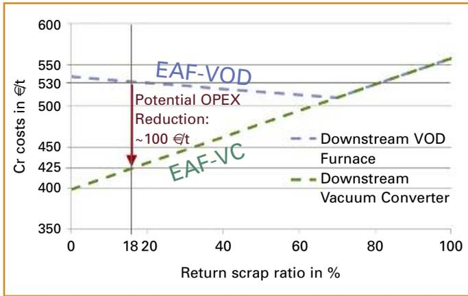
Further potential for savings can be generated in the upstream electric arc furnace. The decarburization speed in the vacuum converter is several times higher than that in a VOD facility. It is thus possible to use raw materials which have a significantly higher carbon content (e.g. FeCr HC).
