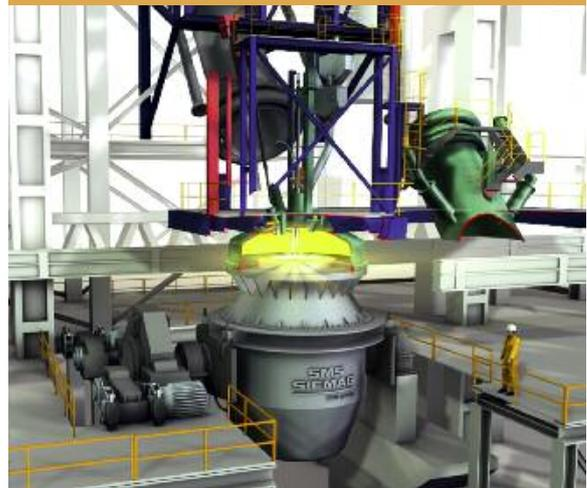
A movable platform is installed above the converter vessel for a fast changeover between atmospheric and vacuum process. Both the exhaust elbow and the vacuum hood are installed on this platform. Instead of transporting the melt between the main decarburization under ambient pressure and the deep decarburization under vacuum, the exhaust elbow is moved and the vacuum hood placed on the converter vessel.
