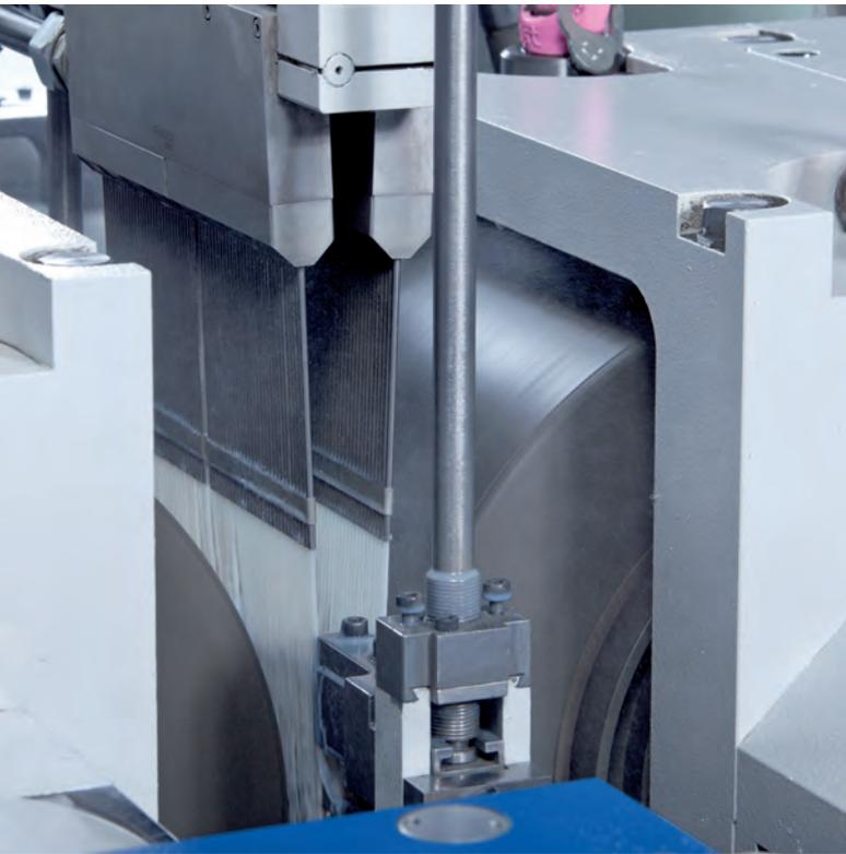
High rigidity, excellent dynamic behavior and low vibrations: these are features the SMS group customers have put their faith in for more than 65 years. All machines operate with a constant grinding axis, dispensing with the need for lateral adjustment of the bar guide and creating ideal conditions for fast, high-quality grinding of bars.
